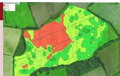
An EC scan of Sandpits shows up a significant area of lighter soil, coinciding with the field's steep undulations, and the Real Results tramlines cut straight through.
