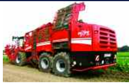
The Grimme Rexor 630 sugar beet harvester: offset wheel positioning gives total surface coverage.
