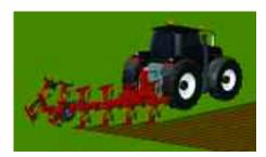
Kuhn has developed a hydraulic system that raises and lowers individual plough blades to create a totally straight furrow edge.
