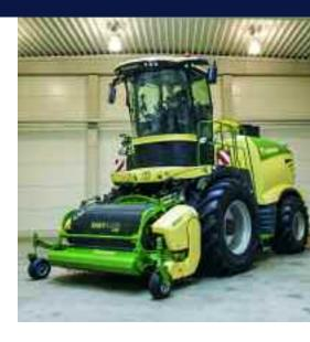
LiftCab raises the cab by up to 70cm to give the operator a clearer picture of work progress.
