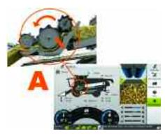
CATS is able to make the various adjustments to produce grain of a consistent quality standard.
