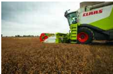
For an easier harvest, wait for the afternoon of a hot day and make sure combine knives are sharp and tight, with no up and down play or wriggling.
