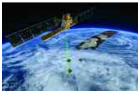
The two new Sentinel-1 satellites (left) can scan the surface of the earth in just six days and use radar (right) to "see" through the cloud layer.
