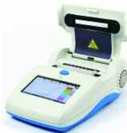
The Genie III device that makes in-field LAMP diagnostics possible.
