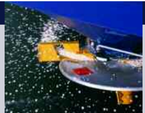
The discs rotate towards each other in the field (left) to provide the greatest accuracy of application. On the headland, the rotation of the discs is reversed (right), with the rear of the vanes creating a sharp headland cut-off.
