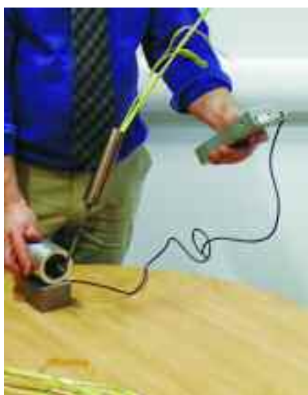
Mitch demonstrates how relative values for stem strength (left) and root anchorage for wheat varieties can be tested.
