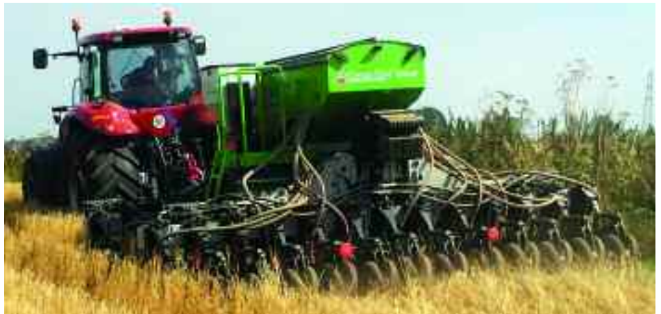
The Cross-Slot drill works straight into the standing stripped straw, with no prior field passes carried out.
