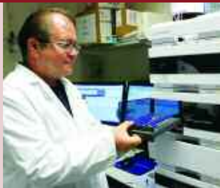
Costin Camarasu loads more samples into the mass spectrometer that separates complex mixtures into its components.
