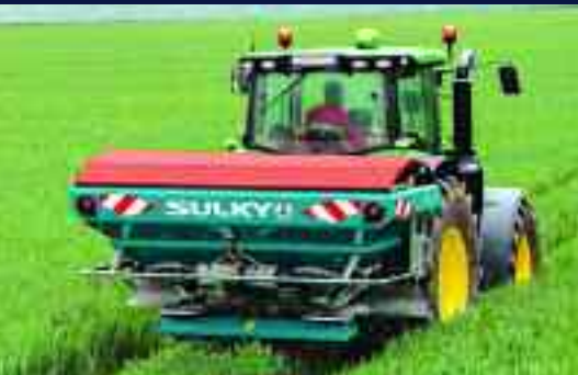
The Sulky X50+ now has two low level sensors and hydraulic drive for the spreading discs.
