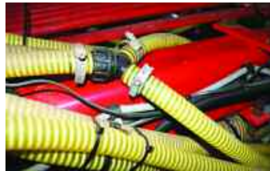
The seeder unit has only eight outlets, with a pipe from one of the central outlets split to make up the nine.
