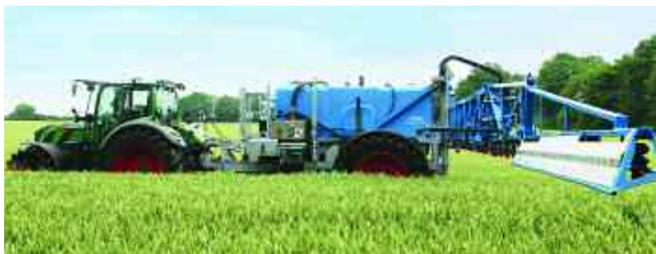
On the Albatross, up to 13 sections of the spray boom can be controlled individually.
