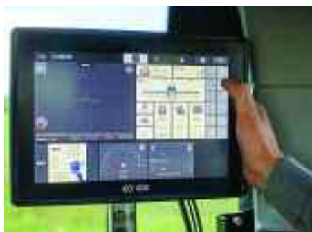
Lemken's new terminal allows you to control two machines through just one screen.
