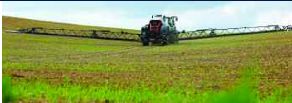
BoomControl Pro on Horsch's Leeb GS has been designed to ensure that the boom stays close to the crop.
