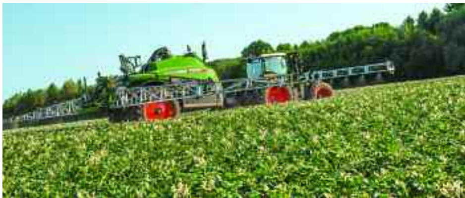
Fendt's new Rogator 300 Series is built around a single-beam chassis.
