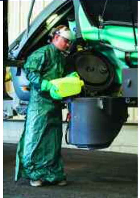
Chemical filling on Vantage Dark sprayers takes place via a newly-designed 35-litre induction hopper.
