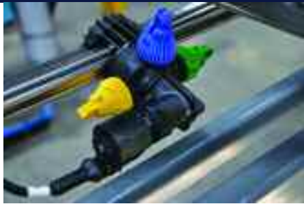
The system means flow can be varied by as much as 70% from a single nozzle type without changing operating pressure.
