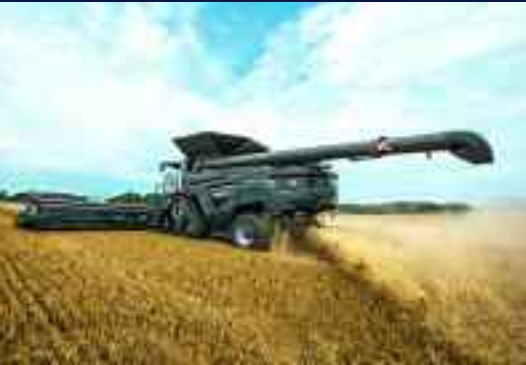
The three-model Fendt Ideal combine line features 4.8m-long rotors – one on the smallest machine, two on the two larger models.
