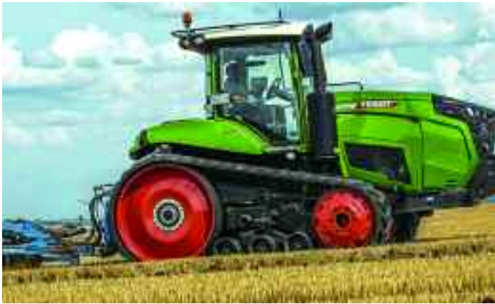
Fendt 900 Vario MT tractors are an all-new blend of the brand's wheeled tractor technology and Challenger tracklayer design.
