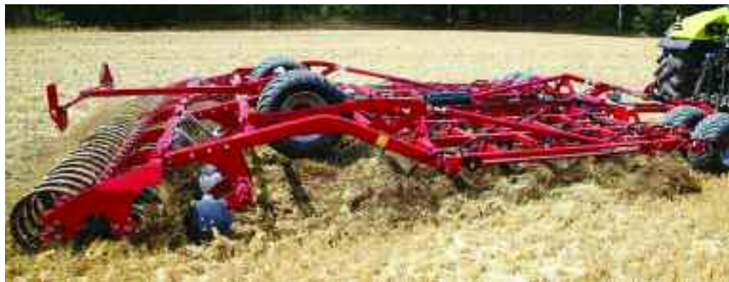
The Horsch Cruiser XL shallow cultivator range features four rows of sprung tines and a rear roller.
