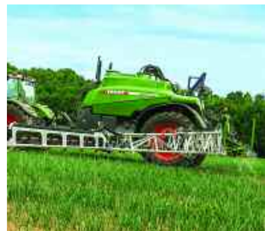
There are four Fendt Rogator 300 trailed sprayers, from 3300-6600 litres nominal capacity and with boom widths from 24-30m.
