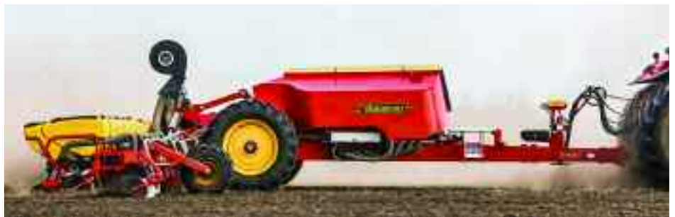
With units set at 500mm spacing, Väderstad's Tempo L precision drill can be used to establish sugar beet and oilseed rape.
