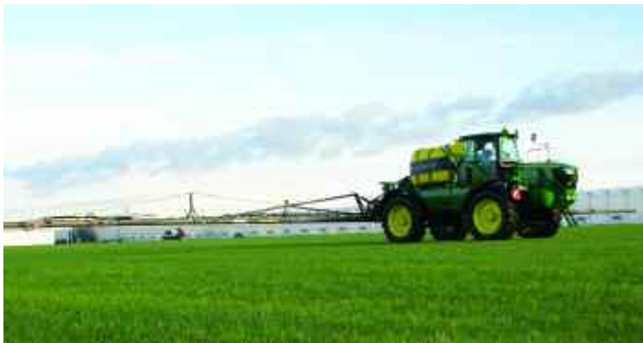
John Deere's R4050i self-propelled sprayer, which joins the R4040i, will be shown equipped with a carbon fibre boom.
