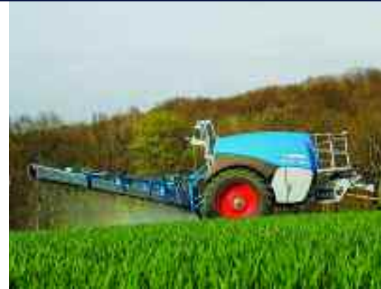
Lemken's Vega 12 trailed sprayer with RA rear-folding boom will be shown with the firm's top specification CCI1200 operating terminal.
