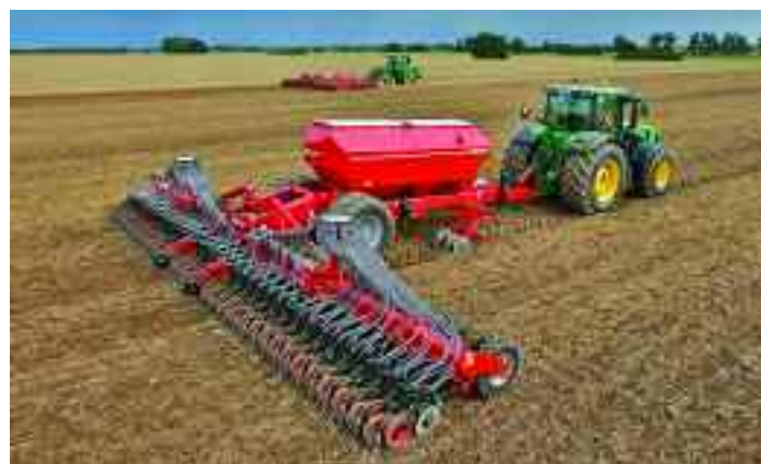
The new 10/12m Horsch Serto SC features an all-over tyre packer combined with a heavy double-disc seed coulters, with two coulters behind each tyre.
