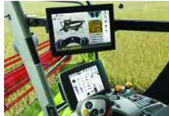
The CEMOS system allows operators to select their desired focus — optimum output, minimum losses etc — and the combine then adjusts settings accordingly.
