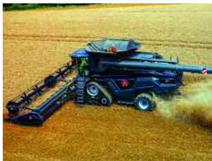
With the new Ideal, Massey Ferguson moves away from hybrid combine design to a true axial threshing and separating system.
