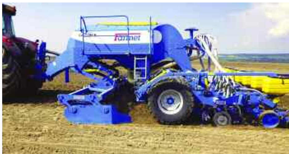
A new 6m grain and fertiliser drill, the Farmet Falcon 600 Pro incorporates leading cultivation elements ahead of fertiliser coulters, consolidation elements and coulters.
