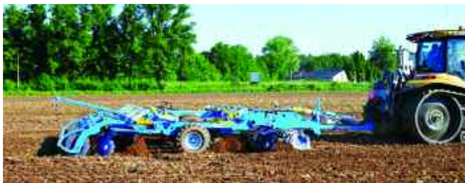
The Farmet Triton 450 is equipped with two rows of 560mm or 620mm discs and two rows of loosening tines spaced at 42cm.
