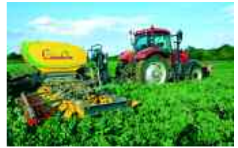
The System Cameleon is used to undersow the grass/clover leys as well as perform inter-row weeding and establish crops as a conventional drill.
