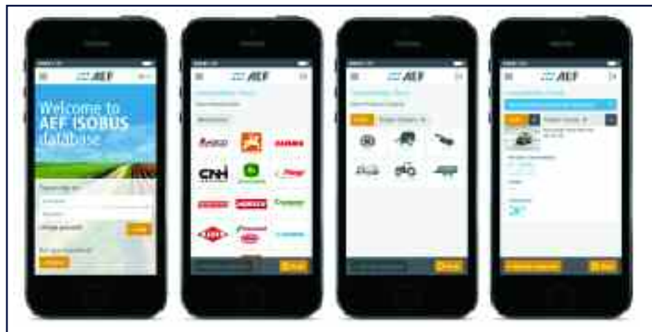
Growers can check the cross-compatibility of ISOBUS-equipped tractors, implements and in-cab devices using the AEF online database.
