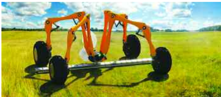
Work is underway to develop a prototype Harry, who will have up to a 1t payload and seed the crop with a punch-planting mechanism.
