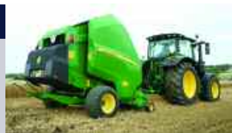
Pretty much new from the ground up — the John Deere V451M mid-range baler rolls up packages up to 1.6m in diameter.
