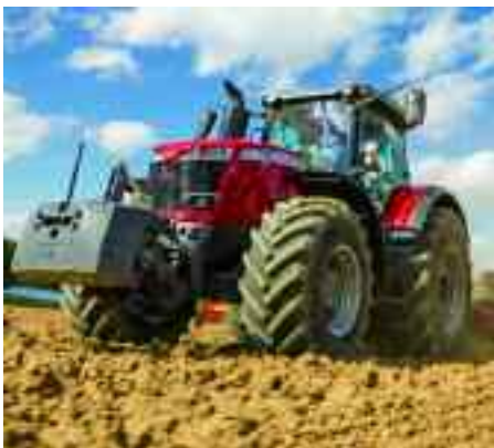
Sufficient ballast is needed to achieve optimum traction, but less is needed as working speeds increase.
