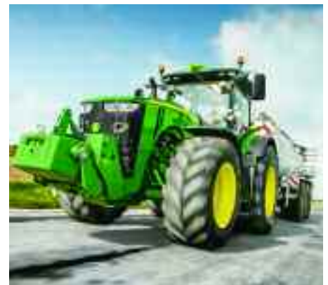
Stripping tractors of ballast when it's not needed saves fuel and tyre wear by reducing overall weight – linkage-mounted ballast blocks make that easier.
