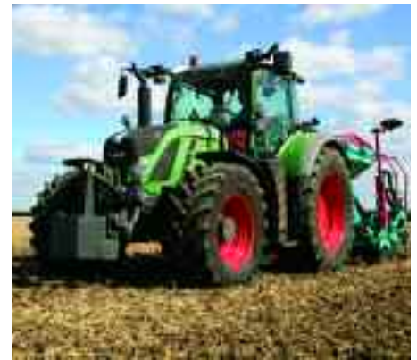
Fendt 724 Vario weighing 8000kg bare needs 7800kg of ballast to get its tyres – Trelleborg TM800 in this case – working at optimum performance for heavy tillage at 6.5km/h. In this application, countering the weight of the rear-mounted power-harrow seed-drill combination is the main consideration when selecting inflation pressure.
