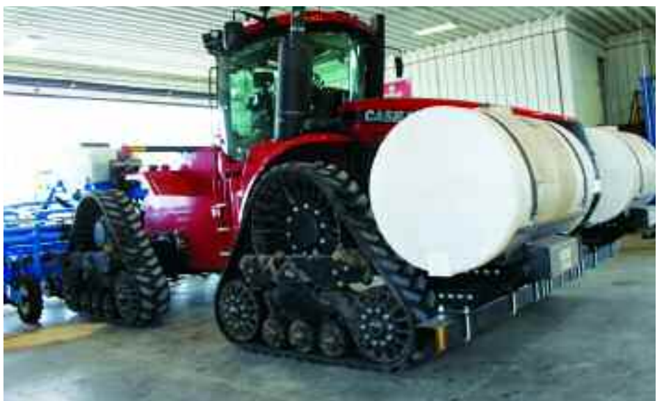
A Rowtrac version of the Steiger Quadtrac is designed to minimise soil trafficking and crop damage in rowcrops.
