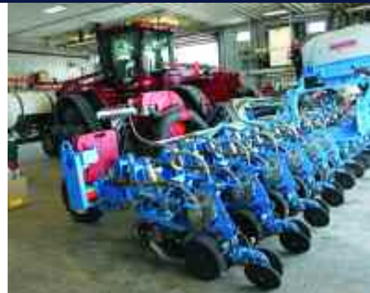
Row-cleaning spider wheels ahead of each seed unit clear soybean trash from coulter paths and prevent hairpinning on this 36-row Monosem seeder.
