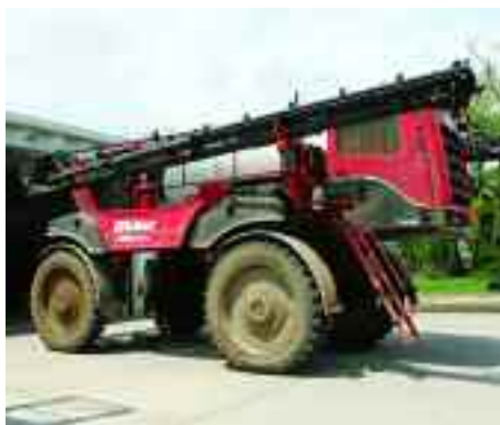
Spraying is handled by this front-boomed 36m Nitro made by Wisconsin firm Miller, part of CNH Industrial since 2014.
