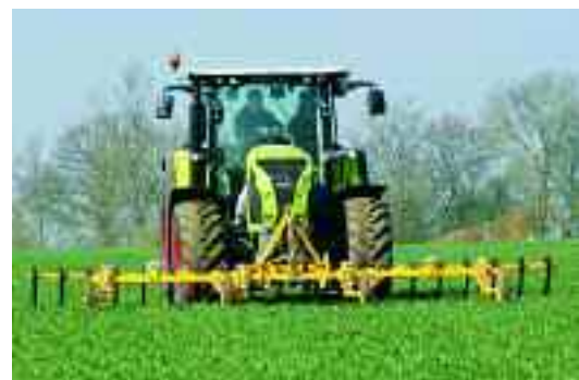
Designed to hoe between strip-tilled rows, Claydon's TerraBlade comes in 10, 14, 16 and 20-row models.
