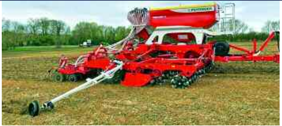
.New 510mm Wave Disc cultivation elements for its Terrasem drills are targeted by Pöttinger at those seeking to work only narrow soil bands.
