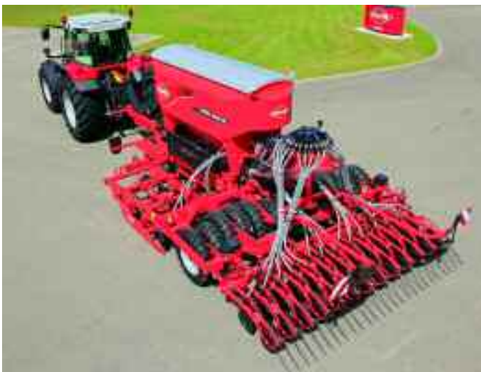
Like other Kuhn Espro drills, the 4000 RC uses two rows of cultivating discs and a row of 900mm offset press wheels.
