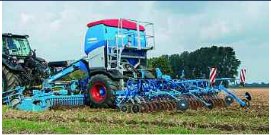
Lemken's Solitair 25 now features automated calibration, operated from the tractor cab using the drill operating terminal.
