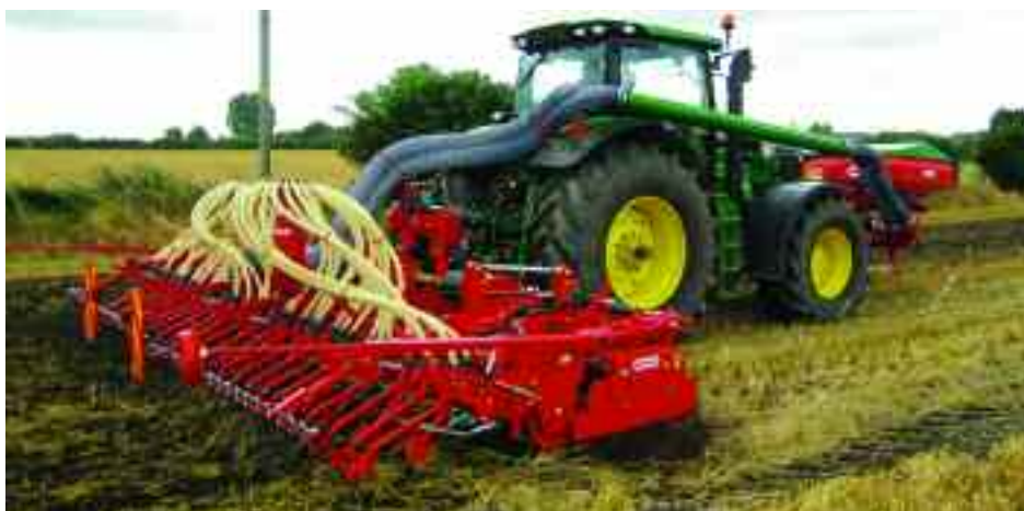
Opico's Maschio Centauro transfers seed from a front-mounted hopper to a rear coulters bar with two or three rows of Suffolk or two rows of single disc coulters.
