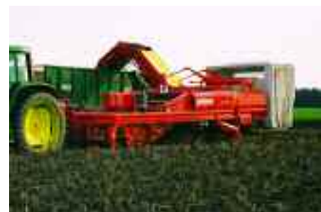
Key for the UK market was a trailed machine with a straight-through separation system.
