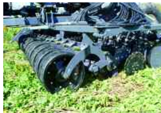
Seed depth on the Sky Easydrill is controlled by the "Tandem" — a rubber depth wheel and two rear press wheels.
