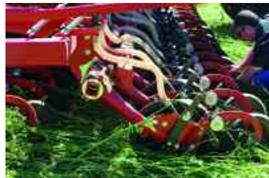
There's up to 310kg of pressure on the SingleDisc coulters, exclusive to Horsch's Avatar, to good soil penetration with very little soil disturbance.
