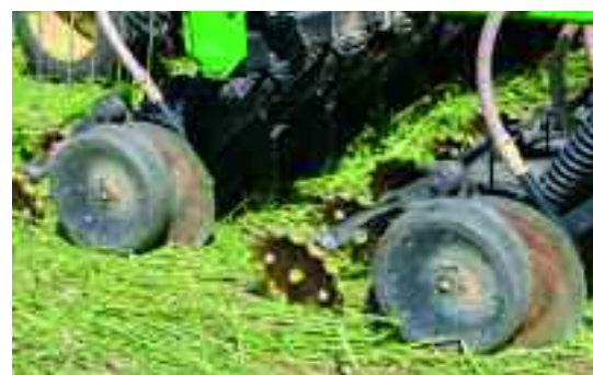
The 7° disc angle on the John Deere 750A allows for precise seed placement in all conditions with very low soil disturbance.
