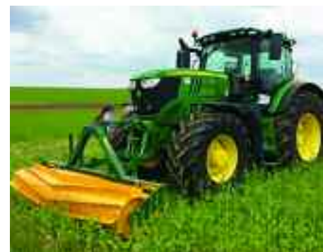
The Cousins crimper roller is fitted with helical blades, rolling over and snapping the crop ahead.
