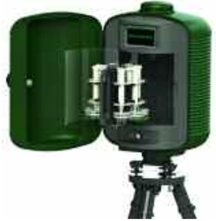
The Fera Spore Sentry prototype is fully automated, simply requiring its reagent cartridge changing once a week.
