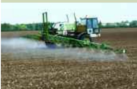
A drift retardant eliminates the very fine and very coarse spray droplets and may be a better alternative to drift-reducing nozzles.
