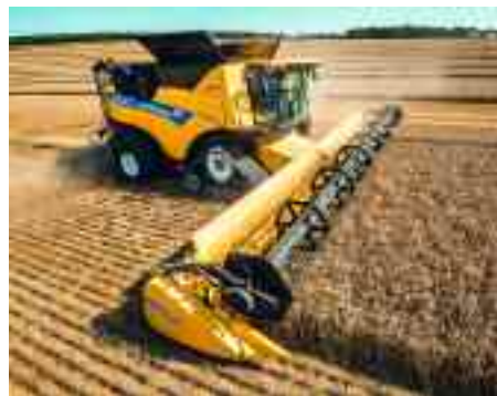
New Holland's IntelliSense allows the driver to choose from four auto-setting strategies: limited losses, best grain quality, maximum capacity or fixed throughput.
