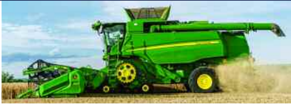
John Deere says the new track system introduced for its 2019 model year combines provides a larger footprint.
