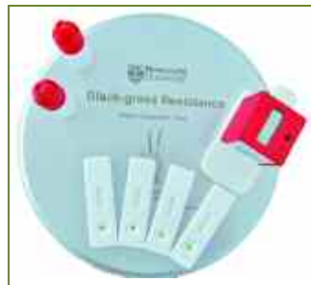
The Mologic BReD diagnostic kit can be interpreted by inserting the device into ‘The Cube’ reader (top right).
