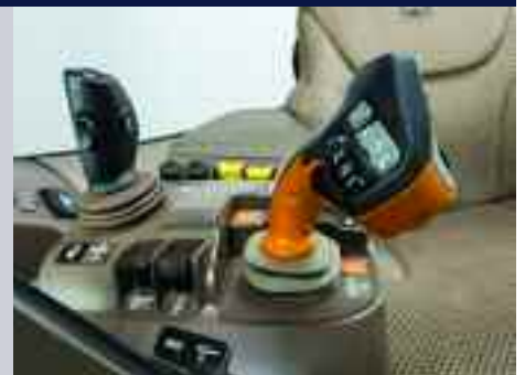
CommandPRO allows the tractor to be controlled from top speed to zero with a simple push or pull of the joystick.
