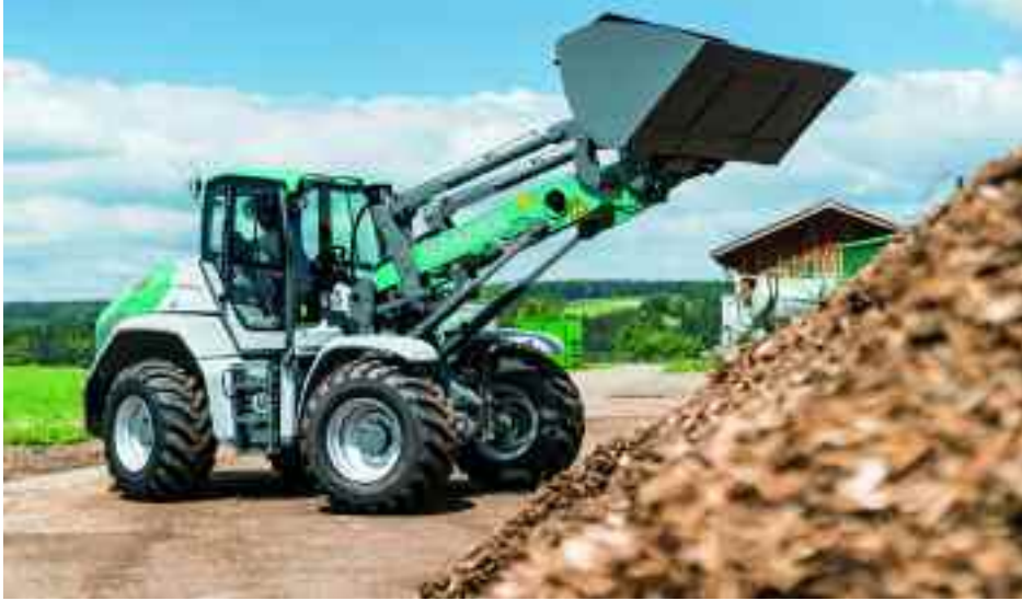
The KL60.8 is Kramer's largest agricultural wheeled loader, with a total weight over 9t and a bucket tipping load of 6100kg.
