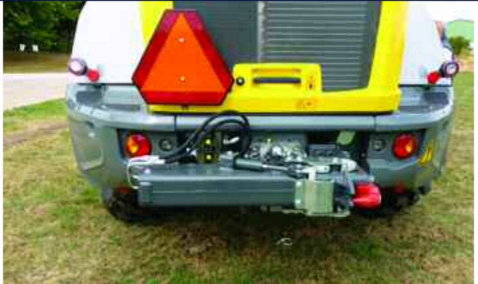
The trailer hitch on the KL60.8 rotates through 90° to improve ground clearance.
