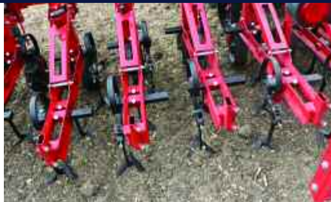
Cameras on the front of the hoe detect the crop row, keeping the hoe blades on track between rows of any crop from field veg to cereals at a forward speed of up to 16km/h.
