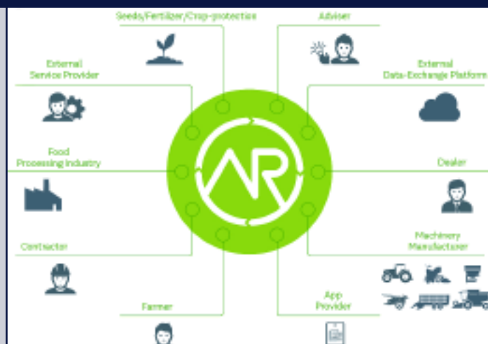
Each user puts together their own personal Agrirouter and defines rules about who exchanges which data with whom to what extent.
