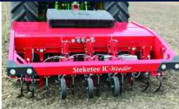
Developed with Wageningen University, cameras mounted under the hood of the weeder detect the individual plants and adjust the line of hoes which snip in between each plant at a forward speed of about 5km/h.
