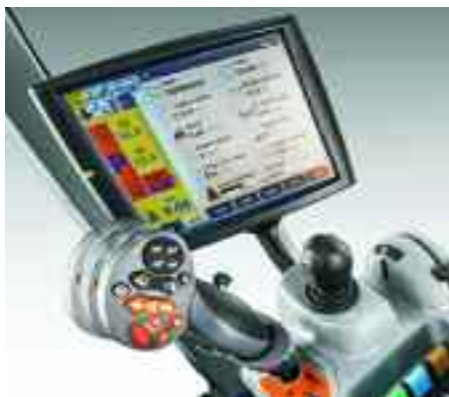
Like other New Holland transmissions, Dynamic Command is operated using the seat-mounted force-response control stick.
