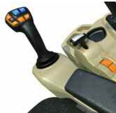
Dyna-6 is controlled by a small 'T' handle on Essential-spec MF tractors (left) and by moving the multi-function lever on Exclusive-spec versions.
