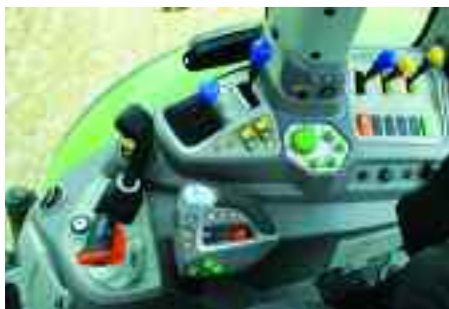
The lesser version of the semi-powershift transmission in Deutz-Fahr 6 Series tractors has button shifting on a range gear lever.
