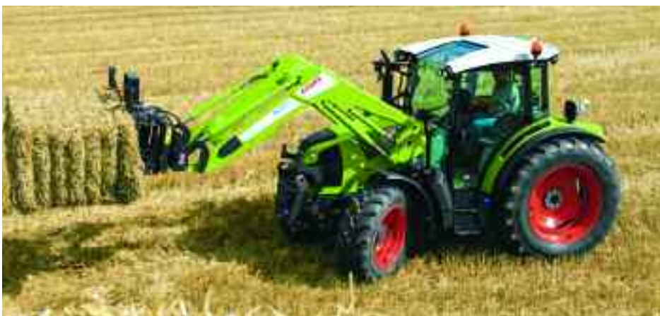
In its latest form, QuadriShift on the Claas Arion 400 Series has gained Smart Stop clutch operation through the brake pedal.
