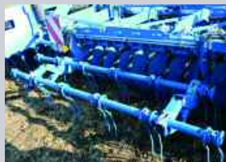
An option on the front of the semi-mounted Rubin is a straw harrow with overload protection.
