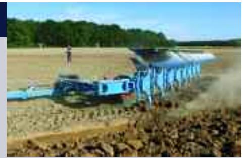
OptiLine, available during in-furrow ploughing, compensates lateral pull arising from the plough's asymmetrical position behind the tractor.
