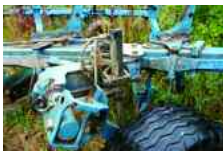
The hydraulic ram for depth adjustment looks a bit small.
