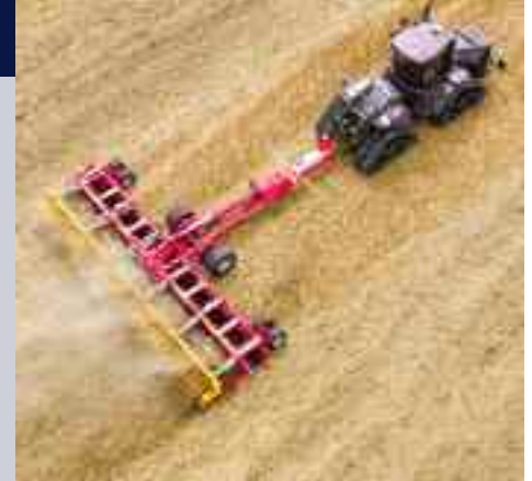
Premiered at Agritechnica last year the Terradisc shallow soil cultivator is now available in working widths of 8m and 10m (pictured).
