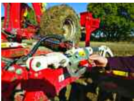
The rear roller is on hydraulic rams set from the tractor seat, and 5mm spacer plates are brought in to fine-tune the depth control.
