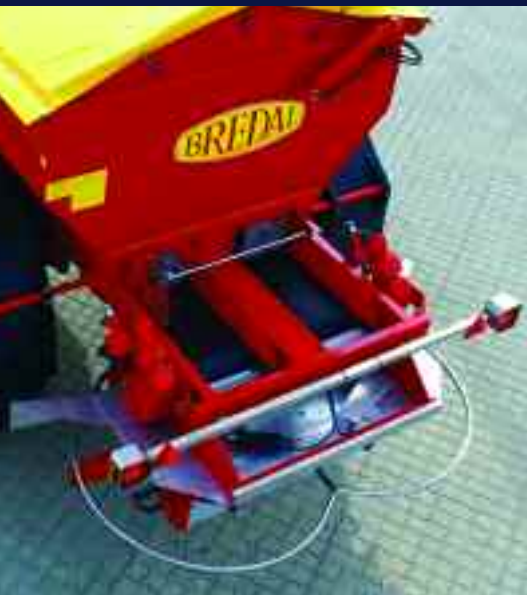
Bredal F Series spreaders have one feed belt per disc so that the delivery rate can be adjusted when section control is being used.
