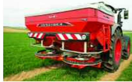
An array of 27 radar sensors arranged beneath each disc monitors the flow of fertiliser off the spreading vanes, enabling software to analyse and adjust the pattern.
