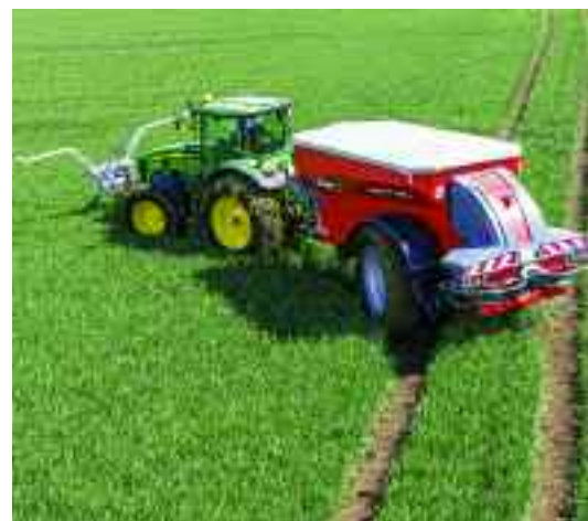
The Kuhn Axent trailed dry spreader is available with separate granular and powdered material application packs.
