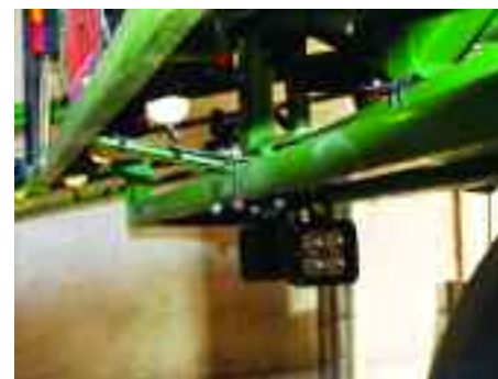
Fitting LED lights to his sprayer's boom has been a low-cost way of improving nozzle visibility when spraying early or late in the day.
