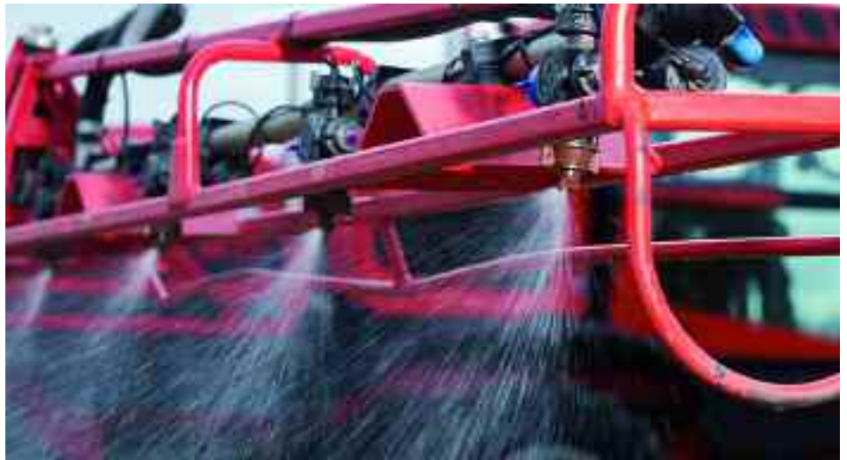
The best pre-em application practice involves a 50cm max boom height, a speed under 12km/h, 200 l/ha water volume and 90% drift reduction nozzles.
