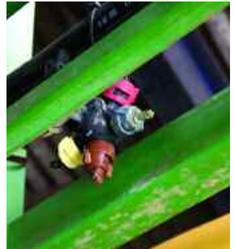
Five-way nozzle bodies allow a quick changeover between jobs.
