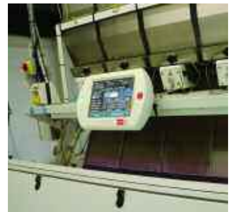
The colour sorter sifts through grain at up to 20t/hr and selects out individual items of a dubious colour as they pass over a cascade.
