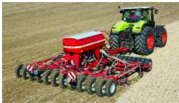
The Duett double seed row wing tine coulters features on the Horsch Sprinter.
