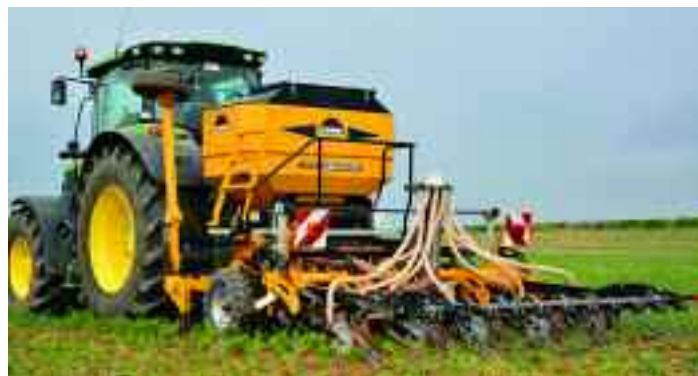
The tractor-mounted Seedaerator can be equipped with a staggered row of flat trash-cutting discs or a soil-loosening tine.
