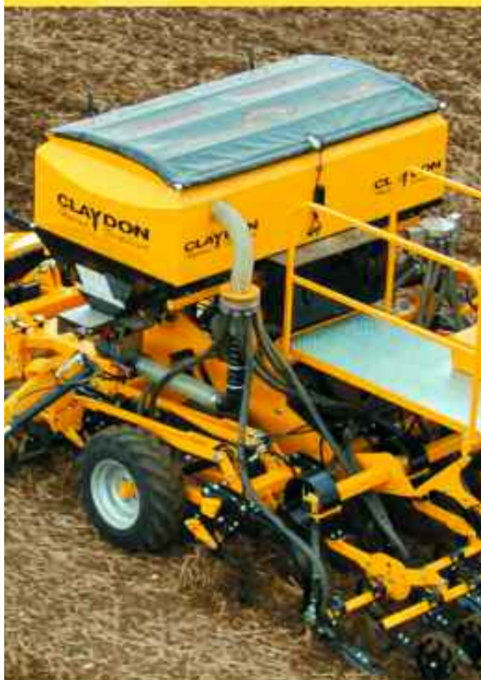
The tractor-mounted Seedaerator can be equipped with a staggered row of flat trash-cutting discs or a soil-loosening tine.
