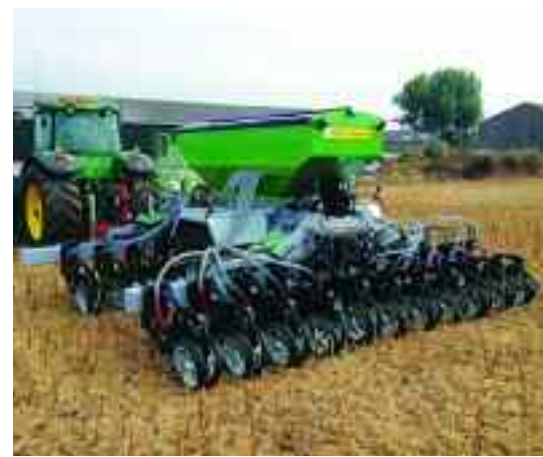
The trailed Cross Slot drill deploys two rows of Baker inverted 'T' coulters, each located alongside a notched disc.
