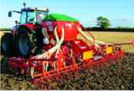
The Primavera is billed as a low-cost seed drill for min-till systems.
