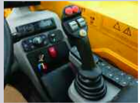
By moving the plethora of dials, switches and buttons to the armrest and screen, it makes for a cleaner, less jumbled cockpit.
