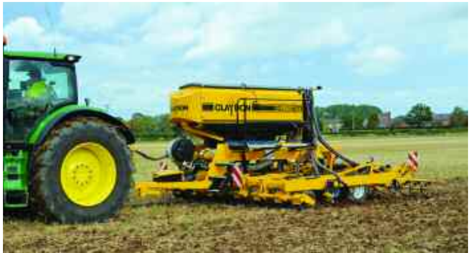
Drilling is carried out using RTK guidance to an accuracy of 2.5cm, allowing him to put spring barley between cover crop rows, while second and third wheats are also inter-row sown.
