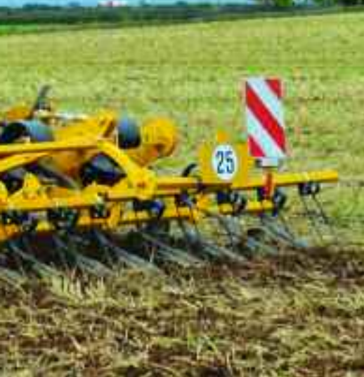
Drilling is carried out using RTK guidance to an accuracy of 2.5cm, allowing him to put spring barley between cover crop rows, while second and third wheats are also inter-row sown.
