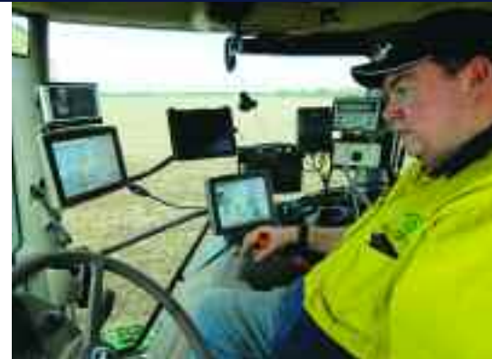
The ITEC system, controlled through a screen on the corner post of the cab, ensures absolute accuracy and reduces driver fatigue.
