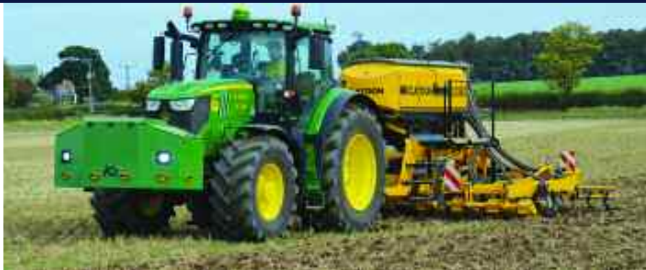
The 215hp John Deere 6125R is used to pull the 4.8m Claydon Hybrid drill at 10-11 km/h, covering the farm comfortably in just four days.
