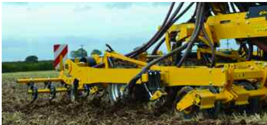
The new 4.8m Claydon Hybrid trailed drill features front shouldered discs, which allow it to work effectively directly into cover crops.
