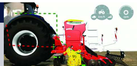
A camera mounted between the power harrow and seeder unit gauges the roughness of the soil surface used to adjust forward speed and PTO revolutions.
