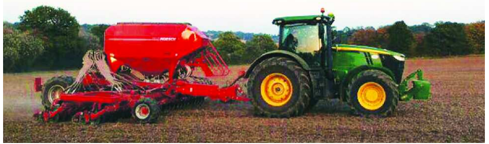
With its staggered single-disc coulters arrangement, the Hunters can usually pull their 8m Horsch Avatar with a 290hp John Deere 7290R.
