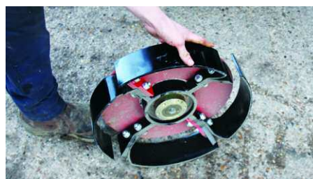
On heavy soils, steel press wheels with four sections and an open centre have proven to produce good slot closing and minimal blockages.
