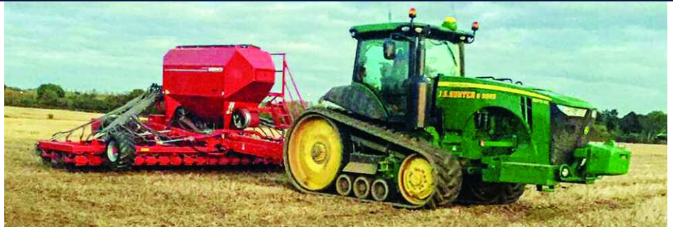
A John Deere 8370RT is available for situations where steeper land, the heaviest soils and wetter conditions are an issue, but it is used minimally.
