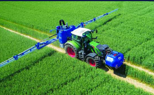
The Lemken Sirius 12 has electric single-nozzle valves which can be operated individually.
