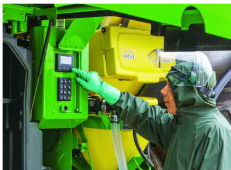
John Deere's 4640 touchscreen display has built-in variable rate capabilities.
