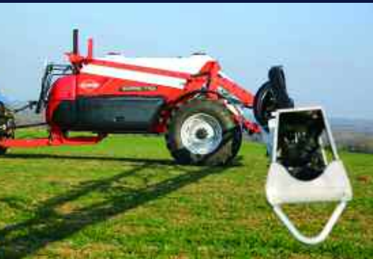
With a 7700-litre tank, the Oceanis is available with compact, all-aluminium booms in widths of 24m to 48m.
