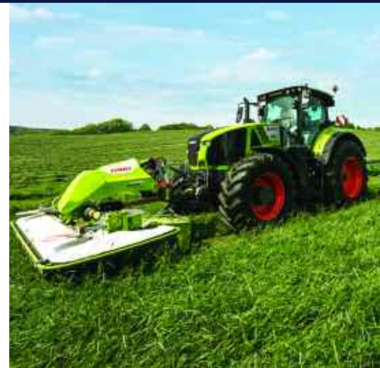
The Disco Move is able to move over a range of 1000mm independent of the tractor linkage to allow for contouring on uneven fields.
