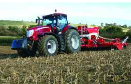
The X8 VT-Drive is McCormick's top model and has either a 157-litre or 212-litre/min variable output piston pump.
