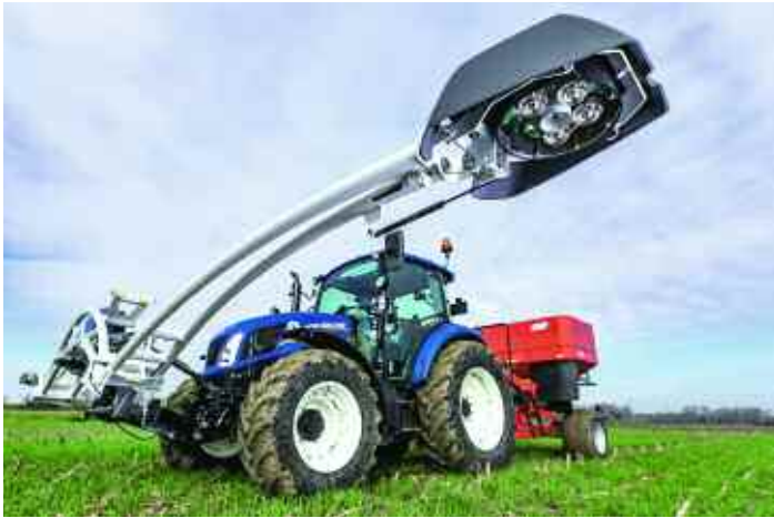
The CropXplorer is a biomass sensor to determine fertiliser rates based on crop needs.
