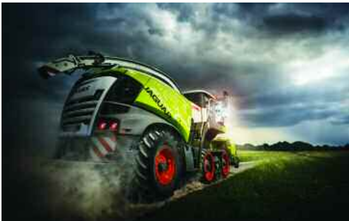
The Claas Jaguar Terra Trac, which adopts the rubber tracked crawler system that has been used on the company's Lexion combines.
