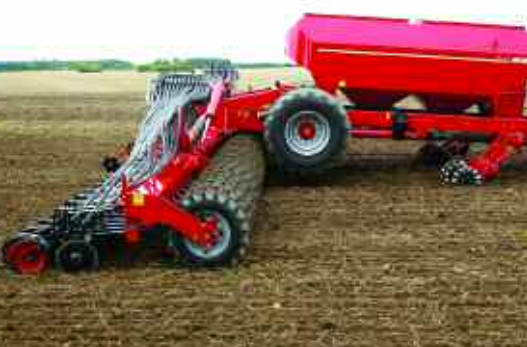
The Serto SC compact seed drill for large farms with working widths of 10m and 12m.
