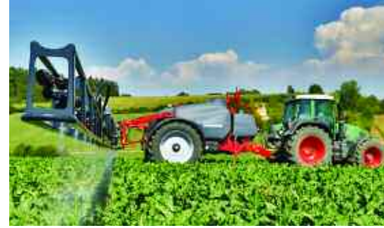
The Leeb 4 AX trailed sprayer is equipped with Horsch's BoomControl Eco system.
