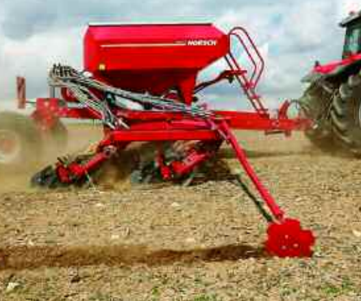
Due to the Avatar's high tare weight, the new single disc coultter is designed for direct seeding.
