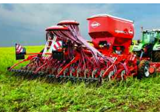
The Aurock triple disc seed drill can establish crops under cover in both min-till and direct drilling conditions.
