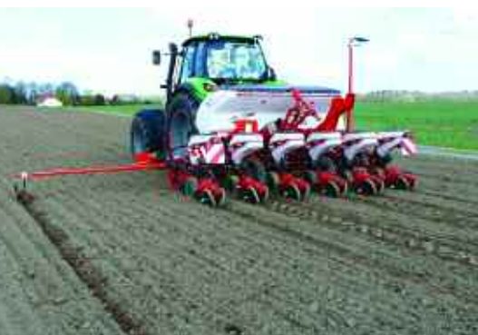
Using an improved seed selection and ejection system, the Maxima 3 allows for accurate seed placement at working speeds of up to 6.2mph.
