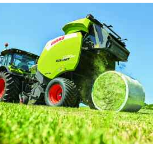
The Rollant 540 fixed chamber round baler features new rollers and a stronger chassis, with the choice of net or film wrapping.
