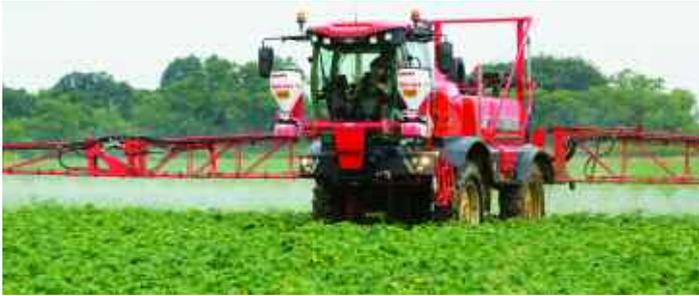
*Crusade has been engineered to reduce drift and aid even deposition of blight fungicides throughout the canopy.*
