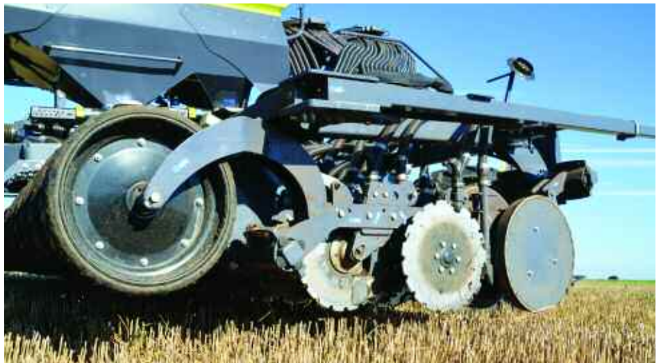
Serrated disc openers are carried in pairs on individual bogey-type coulter carriages with a rubber press wheel up front and smooth steel press rings at the rear.
