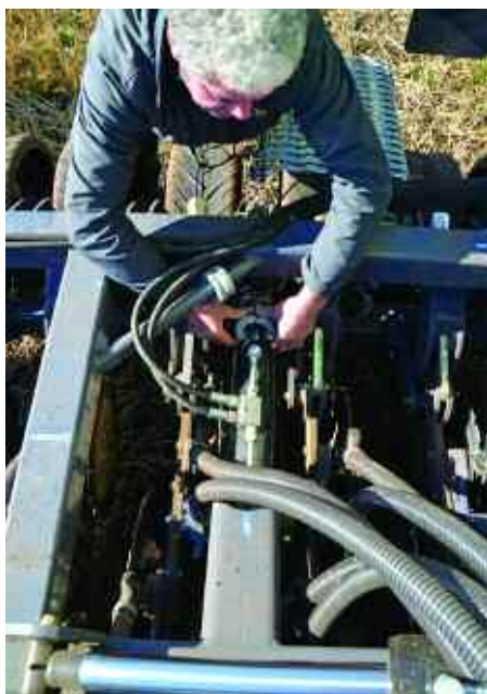
A ram on each wing section sets the fore-aft pitch and weight bias of the coulter carriages to suit soft or hard going.
