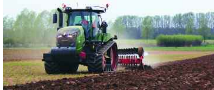
The 943 Vario MT works with a nine-furrow Gregoire Besson plough, an 8m Simba Cultipress and a five-leg Keeble Progressive disc/tine/subsoiler/press cultivator.
