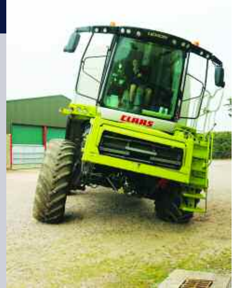
The Montana chassis compensates cross and longitudinal tilt so the combine can deliver the threshing output you'd expect on level ground.
