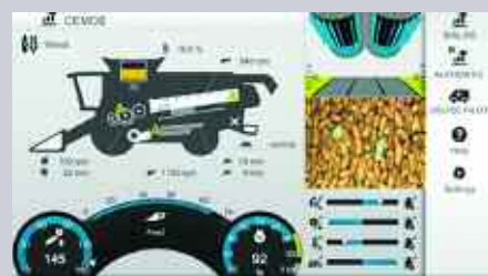
The Grain Quality Camera feeds through real-time pictures of the crop from the elevator and scans these for non-grain constituents and broken grains.
