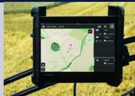
The Fleet View app informs all the operators in a harvesting team about the positions of all the machines and current grain tank fill levels.
