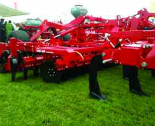
He-Va's CombiDisc can subsoil, cultivate and consolidate in one pass.
