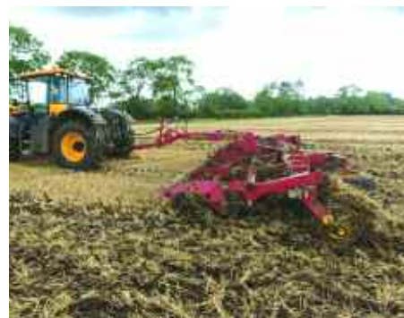
The CrossCutter Disc mulches crop residues without mixing too deep.
