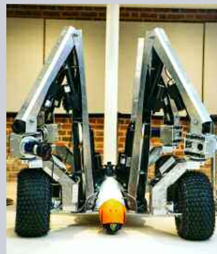
Jack, the prototype of Dick and Harry, first seen at CropTec, has an arachnid, folding design and will soon carry up to a one-tonne payload. Photo: StillVision Photography
