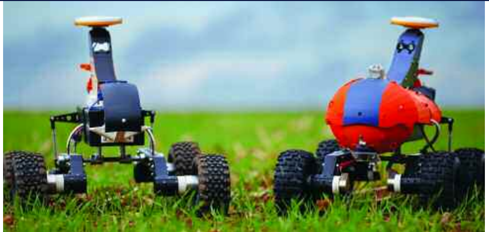
Britney (left) and Rachael – the two prototypes of farmbot Tom who will monitor fields on a plant by plant basis.
